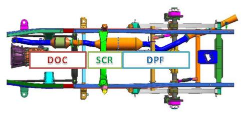
71. This arrangement allows the SCR system to warm up quicker, thus allowing sufficiently reduced NO<sub>x</sub> emissions to pass the cold start test; however, there is a drawback. Because the NO<sub>x</sub> is reduced before the exhaust reaches the DPF filter, there is little Passive Regeneration in the DPF. This, in turn, requires more active regenerations,
