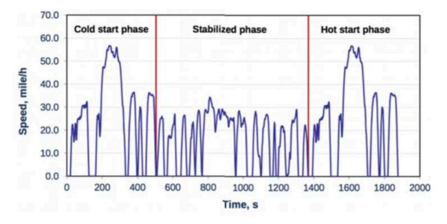
66. Besides urban test cycles such as FTP-75, there are also cycles that simulate driving patterns under different conditions. To assess conformity, several of these tests are carried out on a chassis dynamometer, a fixture that holds a car in place while allowing its drive wheel to turn with varying resistance. Emissions are measured during the test
